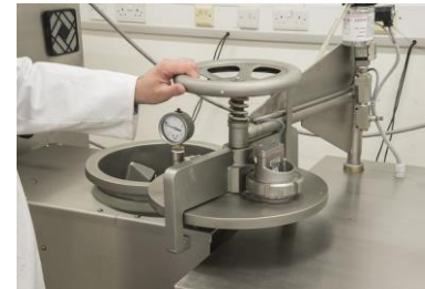
Pressure-vacuum mixing for texture control
