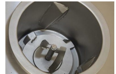
Identical impact plate to production mixers
