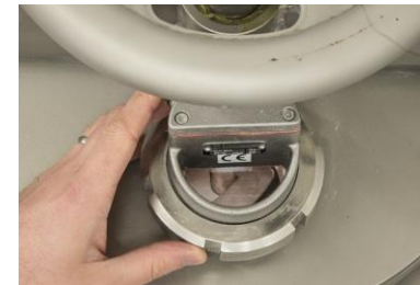
Viewing port and light allows monitoring
