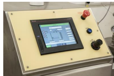
HMI with full process visualisation and recipe control
