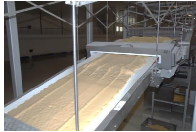
Dough Conveyor with Metal Detector
