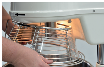
3 Removable rotary stainless steel grid with transparent protective screen
