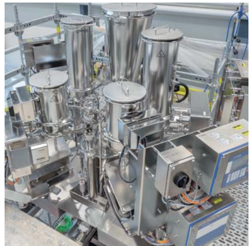
K-Tron Loss-In-Weight Vibrationsdosierer
